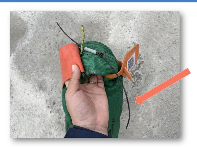
If damage: Optical Fiber No light -> Stop
