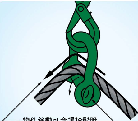
物件移動可令螺栓鬆脫 If the load shifts, the sling will unscrew the shackle pin
