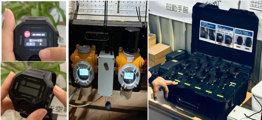
Real-time Gas Detection and Workers' Physical Conditions Monitoring by Smart Watches
