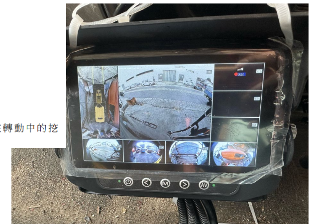
Mandatory application of Mobile Plant Alert System at LPS
