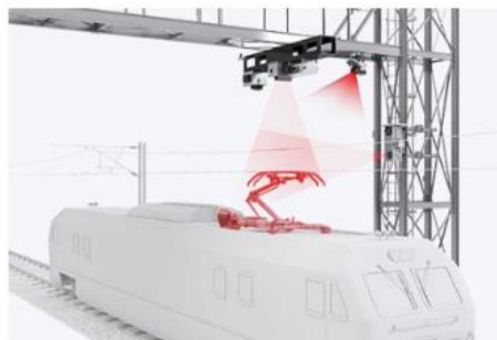
ON-LINE MONITORING OF CONDITION OF TRAIN PANTOGRAPH AND OVERHEAD LINE
