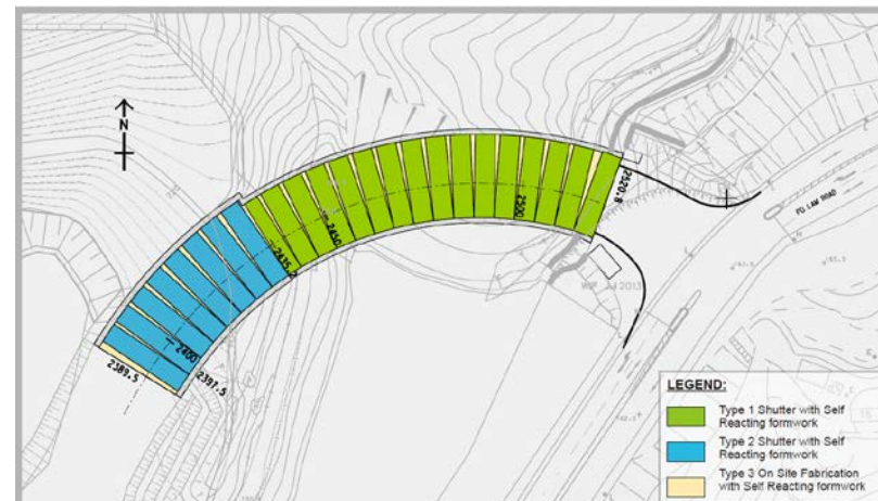
Construction arrangement of permanent lining
