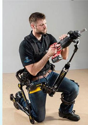
*Exoskeleton to lift heavy tools by transfer its weight to ground from Fortis*
