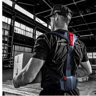
*Upper Body Exoskeleton for Reducing Forces from Strong Arm Technologies*
