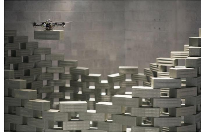
*Drone for architecture installation from ETH*
