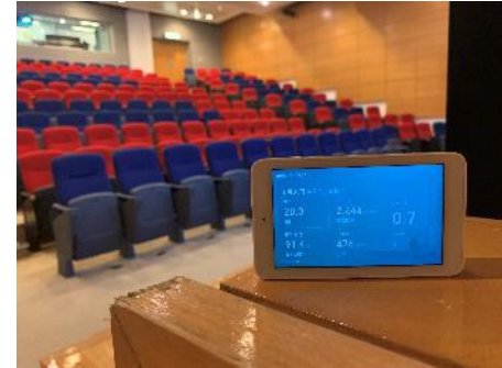
Real time air quality measurement before hand over
